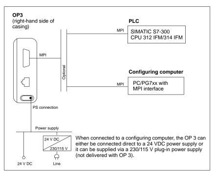
Figure G-1 Point-to-Point Connection (Setup for Configuring the OP3)
