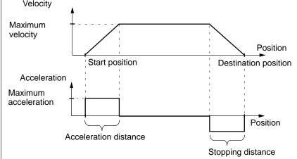
Figure 6-8 Velocity/Acceleration Profile in the Case of Frequency Converters
