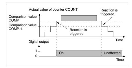
Figure 5-4 Example: Trigger Reactions
