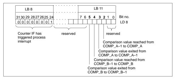
Figure 4-9 Start Information of OB 40: Which Event Triggered Interrupt (Counter IF)?
