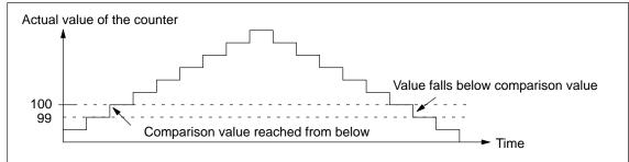
Figure 5-3 Events to which a Comparator Reacts
