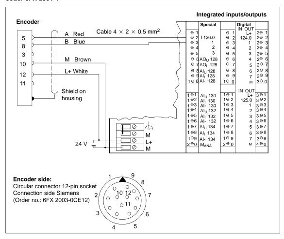
Figure D-2 Terminal Connection Model for Incremental Encoder 6FX 2001-4
