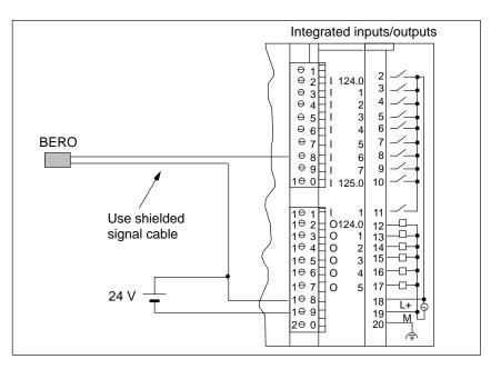
Figure 3-4 Sensor Wiring (CPU 312 IFM)
