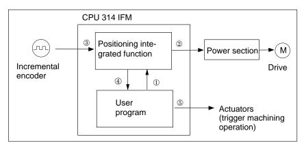
Figure 6-12 Inputs and Outputs of the Positioning Integrated Function
