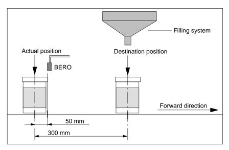
Figure 6-28 Positioning Operation Sequence
