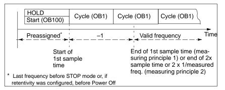
Figure 3-2 Display of First Valid Frequency Value
