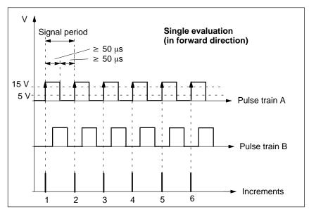
Figure D-1 Pulse Evaluation and Properties of the Counter Pulses
