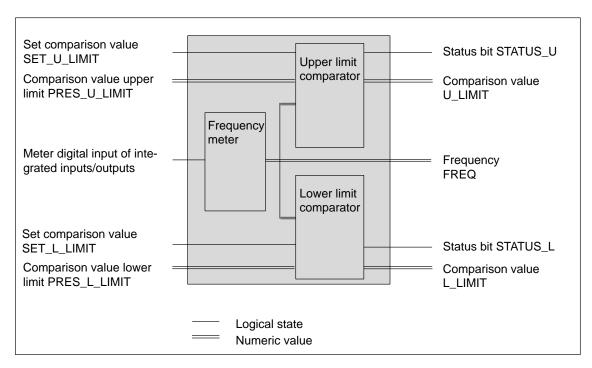
Figure 3-1 Block Diagram for Frequency Meter Integrated Function
