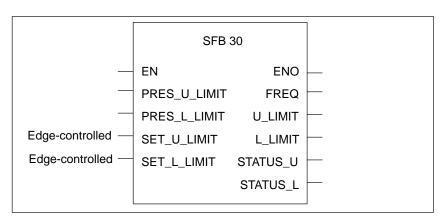
Figure 3-5 Graphical Illustration of SFB 30
