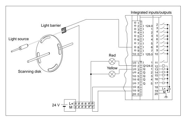
Figure 3-7 Speed Monitoring of a Shaft (1)
