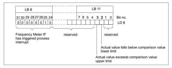
Figure 3-6 Start Information of OB 40: Which Event Triggered Interrupt (Frequency Meter)?
