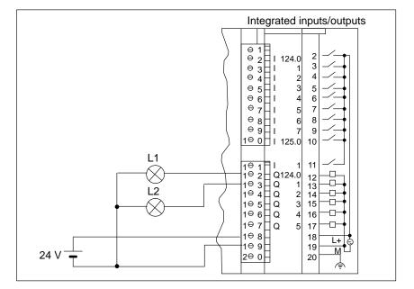
Figure 4-7 Actuator Wiring
