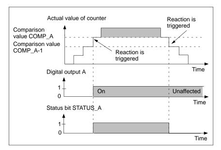
Figure 4-4 Example: Trigger Reactions
