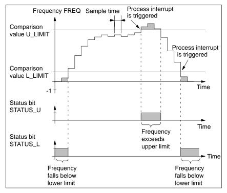
Figure 3-3 Function of the Comparator
