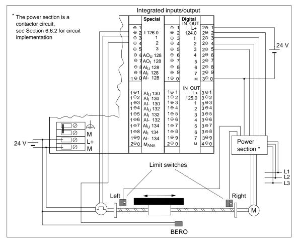
Figure 6-31 Positioning a Worktable
