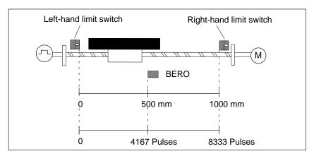
Figure 6-32 Assignment of Distances/Pulses to the Switches
