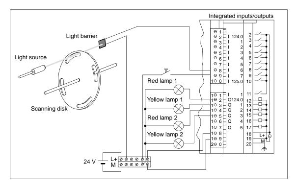
Figure 3-11 Speed Monitoring of a Shaft (2)
