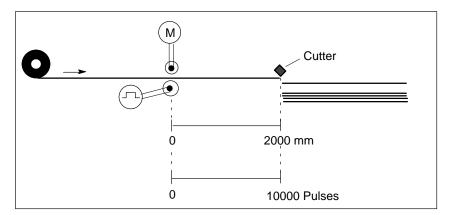
Figure 6-25 Assignment of Distances/Pulses
