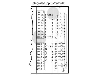
Figure 1-1 Integrated Inputs/Outputs of the CPU 312 IFM for Integrated Functions
