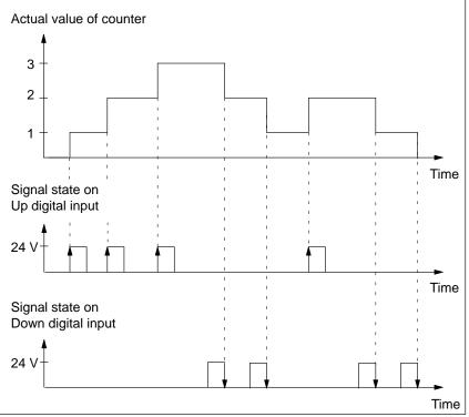
Figure 4-2 Counting Pulses and Actual Value of the Counter
