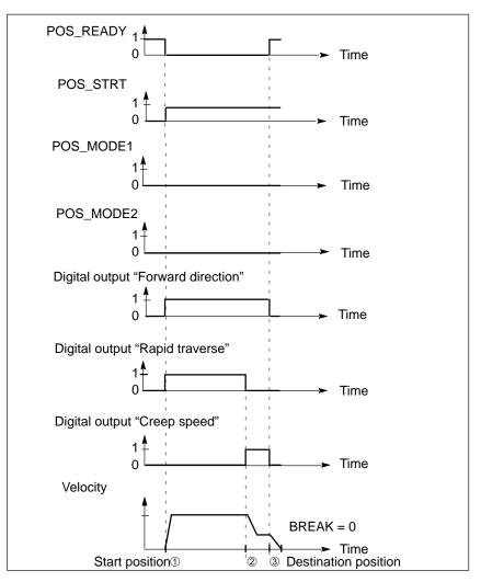
Figure 6-23 Positioning Operation for Rapid Traverse/Creep Speed Drive Forward
