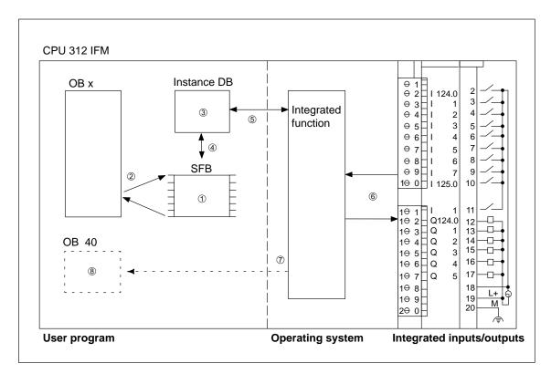
Figure 2-1 Inclusion of the Integrated Functions in the CPU 312 IFM
