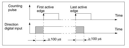
Figure 5-5 Timing of the Direction Digital Inputs for Counters A and B
