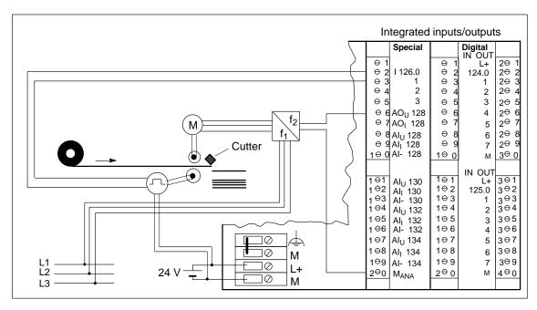
Figure 6-24 Cutting Foil to Length
