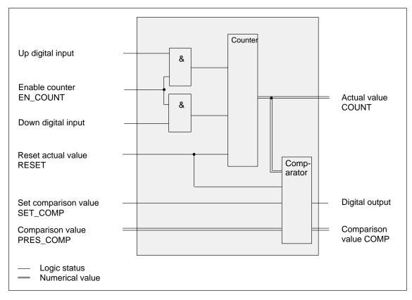
Figure 5-1 Block Diagram for Counter A/B Integrated Function
