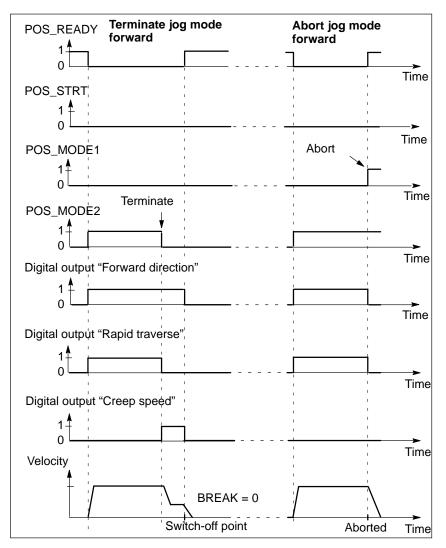
Figure 6-22 Jog Mode Forward and Terminating/Aborting Jog Mode
