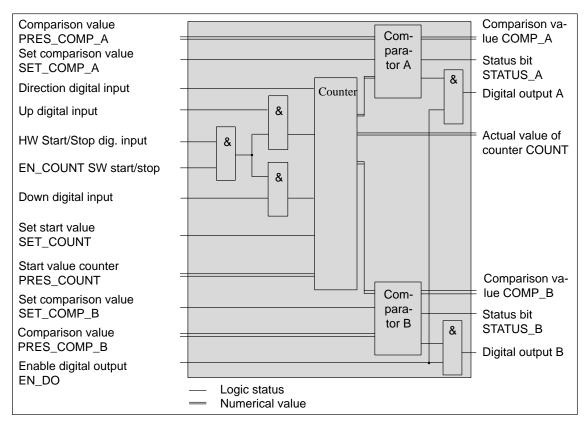
Figure 4-1 Block Diagram for Counter Integrated Function
